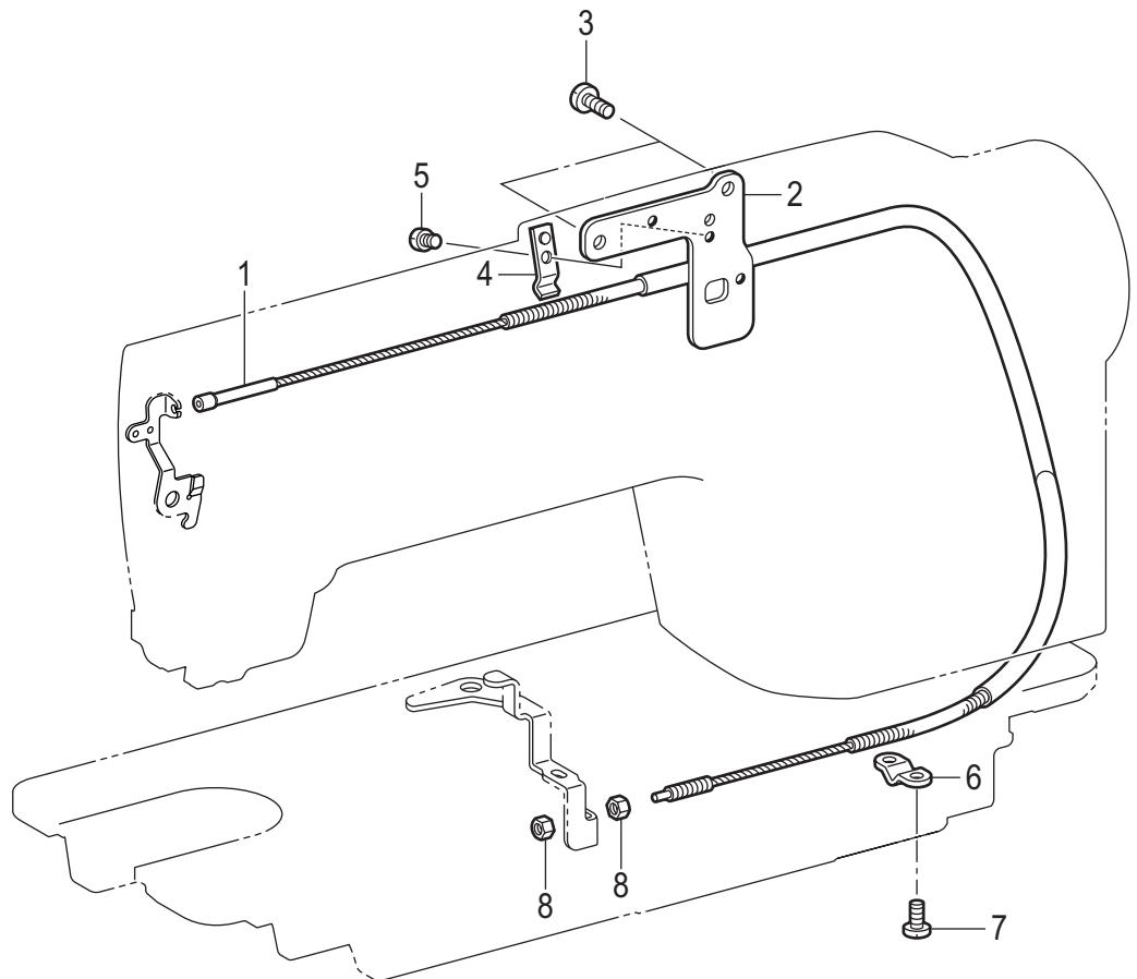
N. 糸緩め関係 / Tension release mechanism
