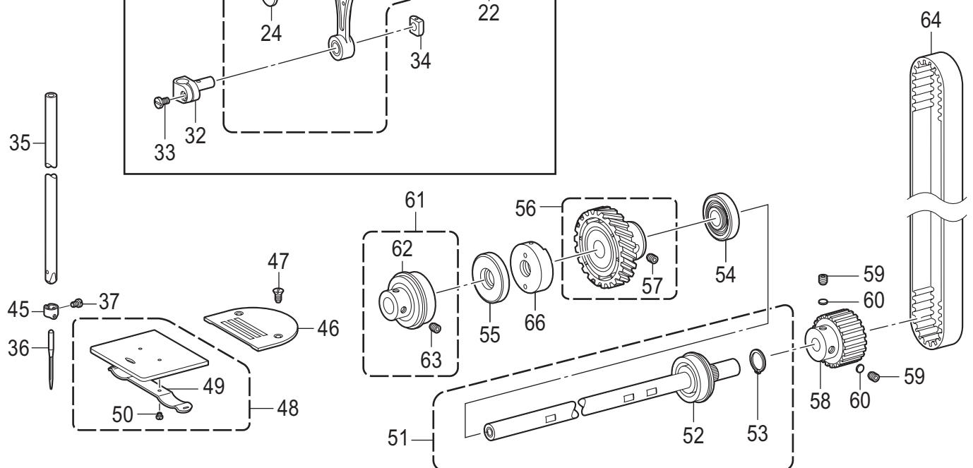
B. 針棒・天秤関係 / Needle bar and thread take-up mechanism
