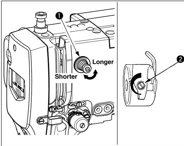
If thread tension controller No. 1 **1** is turned clockwise, the length of remaining thread on the needle after thread trimming will be shorter. If it is turned counterclockwise, the length will be longer. Shorten the length to an extent that the thread is not slipped off.
