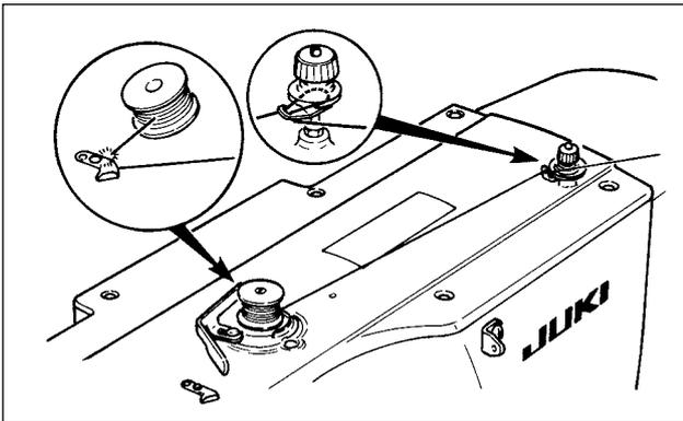
Thread the bobbin winder and wind the bobbin thread onto the bobbin as illustrated in the figure.
