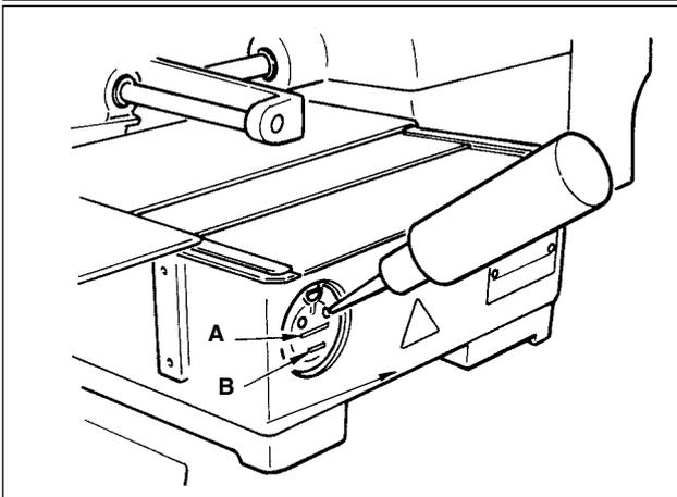
Check that the place between lower line **B** and upper line **A** is filled with oil. Fill there with oil using the oiler supplied with the machine as accessories when oil is short.
