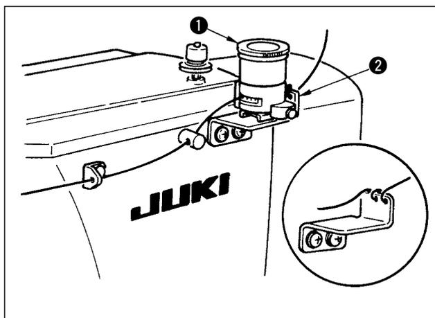
Fix silicon oil tank ❶ (MAXAP30EX00) with the magnet.
