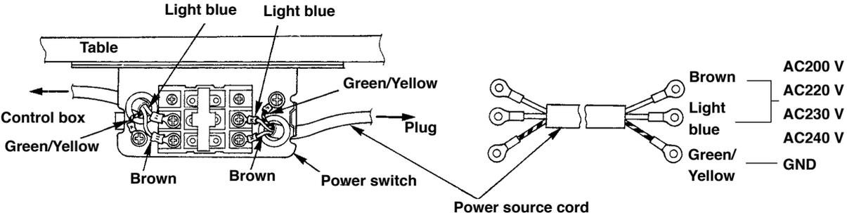
**Connecting three phase 200V, 220V and 240V**
