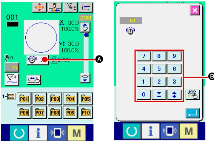
1) Select THREAD TENSION button **A** in the sewing screen.
