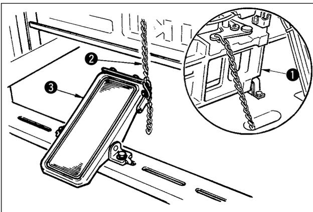
Connect the machine **1** and manual pedal **3** with chain **2**.
