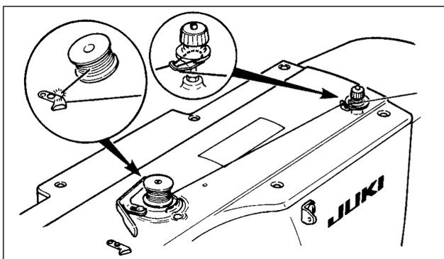
Thread the bobbin winder and wind the bobbin thread onto the bobbin as illustrated in the figure.
