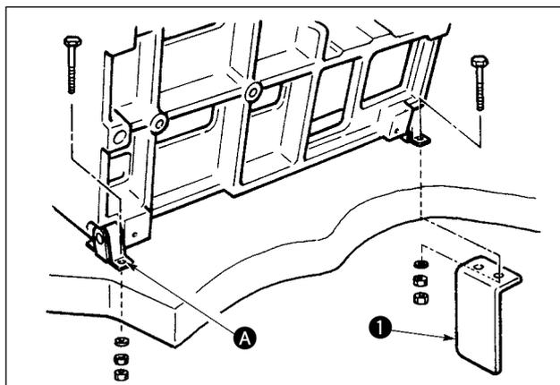
1) Fit the holes of hinges **A** to the holes of table and fix as shown in the figure.
