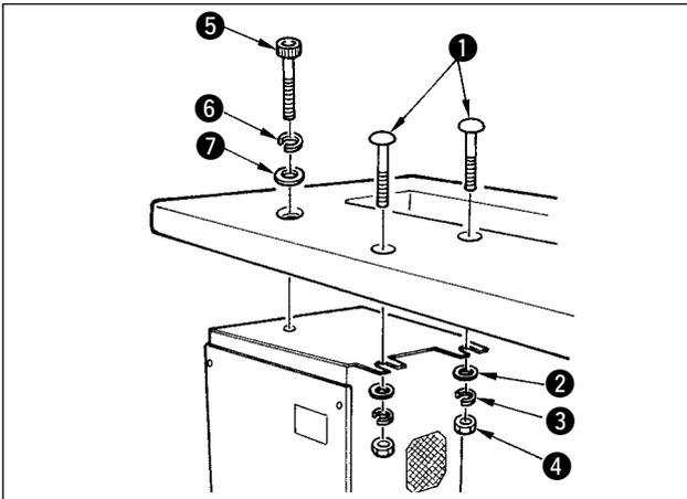
Install the electrical box on the underside of the table at the location illustrated using round-head bolt ①, plain washer ②, spring washer ③ and nut ④ supplied with the machine, and using bolt having hexagonal indentation on the head ⑤ spring washer ⑥ and plain washer ⑦ supplied with the machine.
