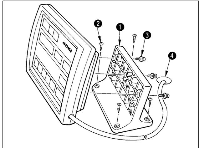
Fix operation panel installing plate **1** to an optional place on the table with wood screws **2**, and pass the cable through table hole **4**. Fix the operation panel on panel installing plate **1** with screws **3** supplied as accessories. Fix the cable on the bottom surface of the table with the staples supplied with the machine as accessories.
