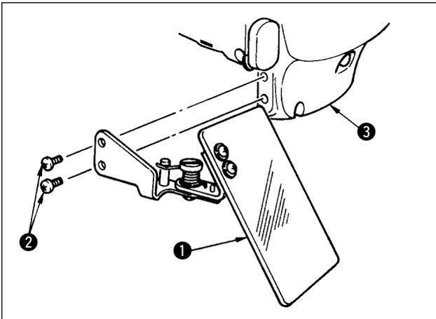
Use eye protection cover ① after securely attaching it on face plate cover ③ with screw ②.
