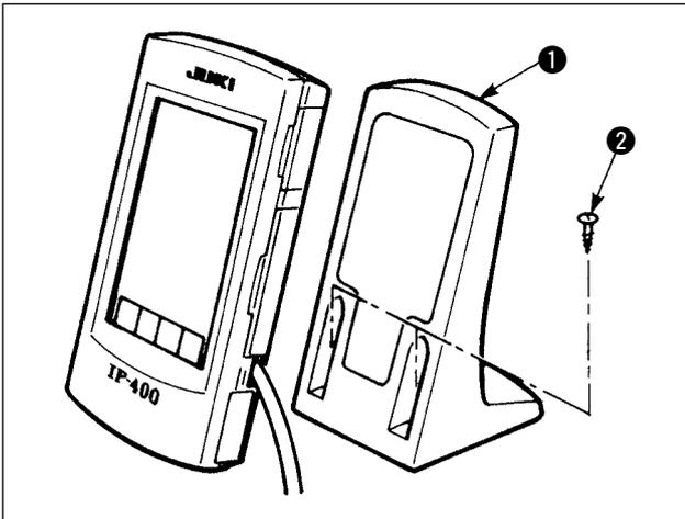
Fix operation panel installing plate **1** to an optional place on the table with two wood screws **2**.
